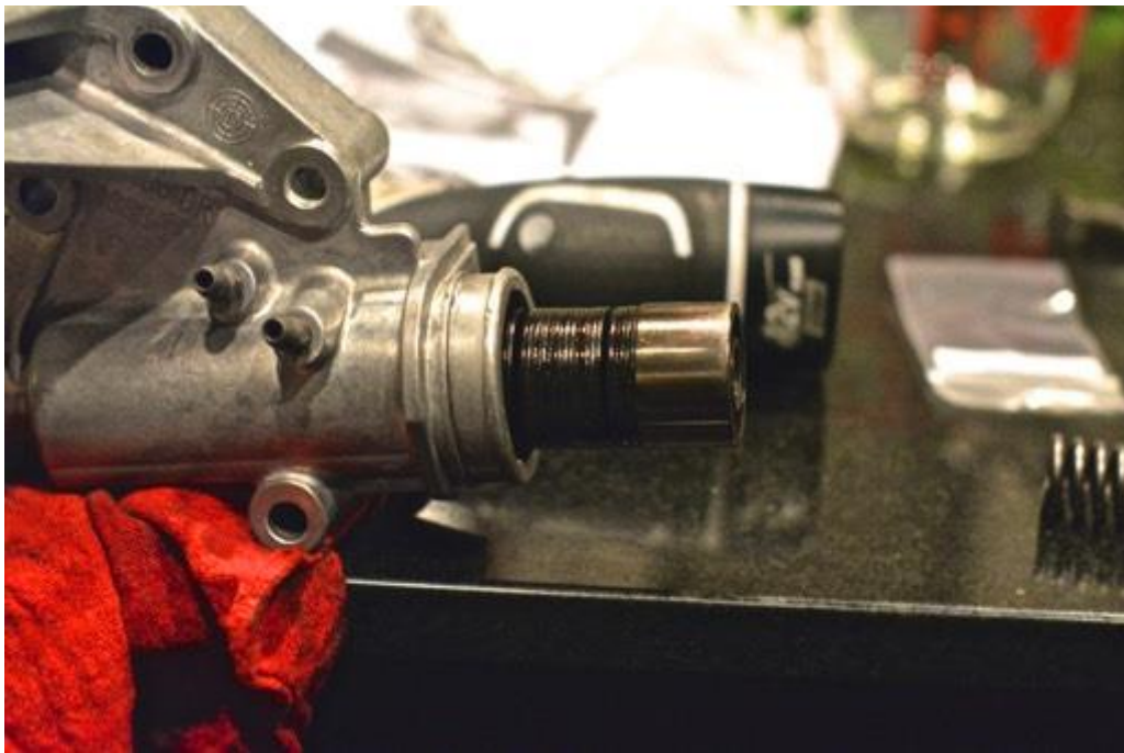
I fitted the new tensioner boot over the plunger and restored the C-clip. I "re-bent" the C-clip because it was a little bit loose.
