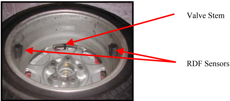
Picture of location of RDF Sensors
