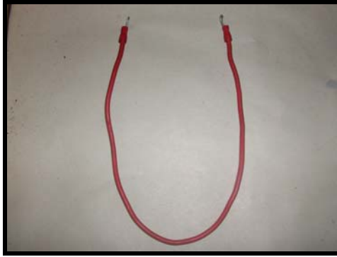
Picture of Relay Jumper Lead
