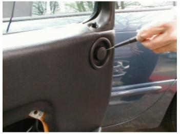
4. Now the doorlock knob needs to be removed. First <u>pry off the cover</u> over the knob with a thin screwdriver (or something similar).
