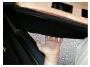
Work your way <u>around</u> the edge of the panel, prying it away from the door (the clips "pop" in and out). In addition to the clips, the panel is held in at the top where it pushes down into place.
