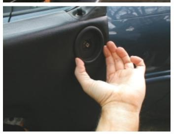
It just <u>screws</u> out. The center of the backing is threaded. If it is hard to get started, you may need to find something that you can insert into the notches in the backing to turn it (I brightened the previous photo some so the notches are more visible).
