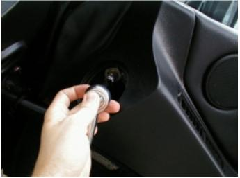
5. Now it's time to start removing some bolts. The panel and armrest are held in by several 10mm hex-head bolts, so you will need a 10mm socket, and an extension for your socket wrench.
