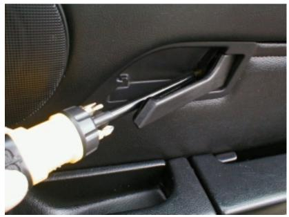
2. Pull the door handle to reveal a <u>screw</u> behind it that holds in the door-handle backing.
