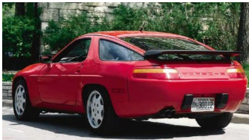
V-8 Porsches had 326 horsepower with manual transmission, 316 with automatic.
