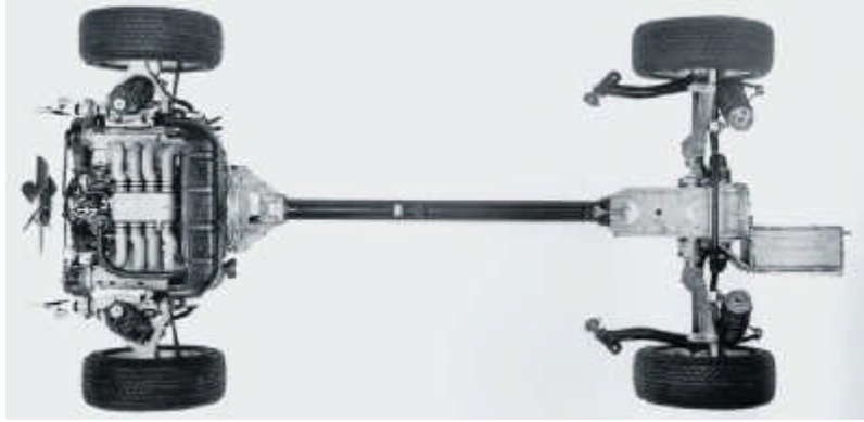
Its novel suspension and mounting structure gave the Porsche 928 great handling.
