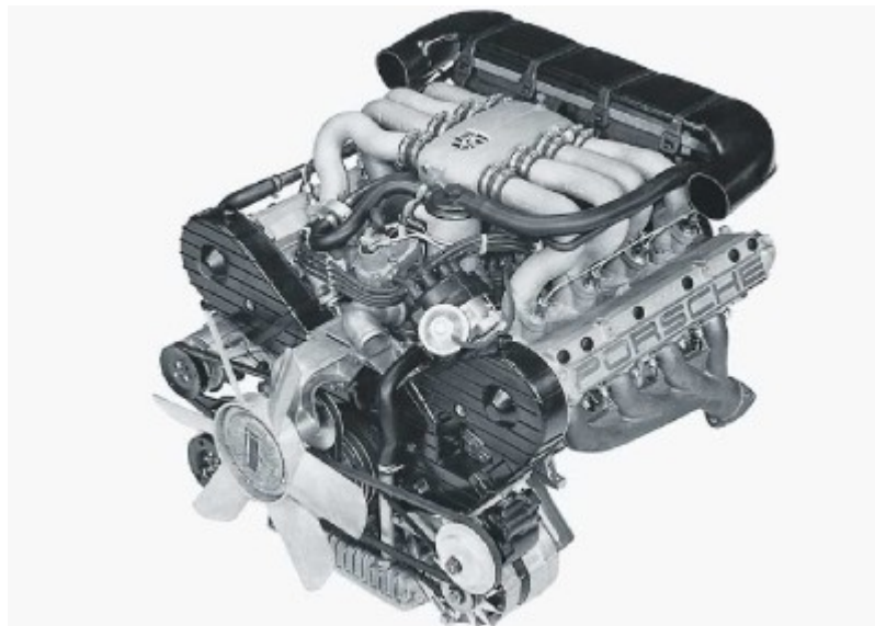
The 928's water-cooled aluminum twincam V-8 was an engineering tour de force.
