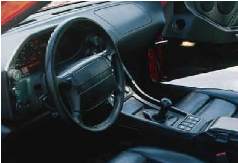
Tilting the steering column of the Porsche 928 also moved the instrument pod.
