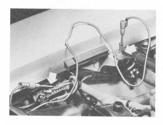
This test could also take place direct on the sensor. Pull off plug on sensor and connect with ground.
