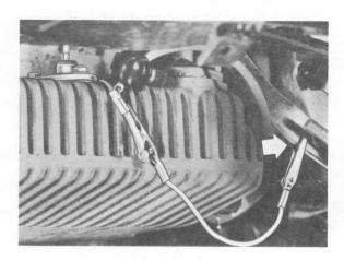
Test on Oil Pressure Switch
