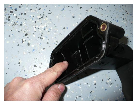
5. Cut the baffles out with a dremel or a die grinder, getting rid of them all the way down the base
