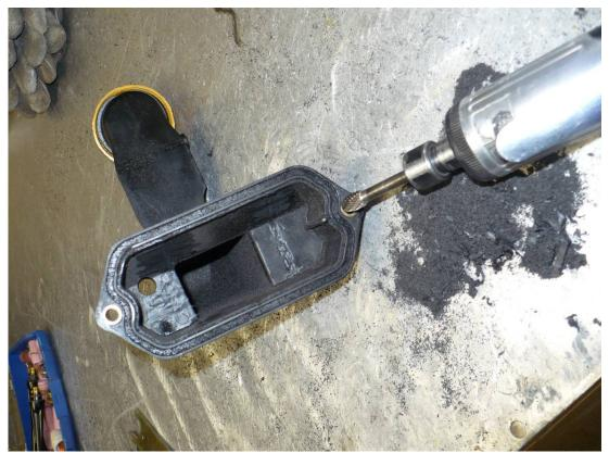
The oil fill/breather box is now ready to be installed over the air/oil separator scrubber box.
