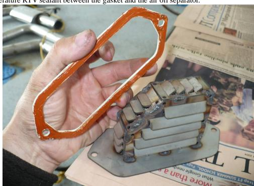
7. Lower the air oil separator over the paper gasket and align the holes of the gasket, separator and engine block
