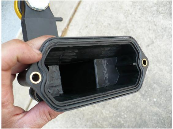
9. Install the oil filler/breather cover over the entire assembly and tighten down the M6 bolts (factory). Do not over-tighten!
