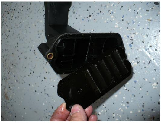
4. The oil fill breather cover must be modified to remove the internal baffles.
