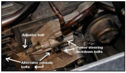
22 - Loosen the air pump 13mm lockdown bolt, and loosen the 13mm adjuster nut. I had trouble getting it to full loose, so I added another nut (M8-1.25) to the adjuster and tightened it to full loose. Remove the belt and mark it "AP".
