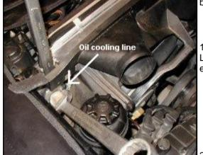
19 - If you loosened the oil cooling line, snug it back together. Later when you hand-crank the engine you could pump enough oil up to spill. (I know!).
