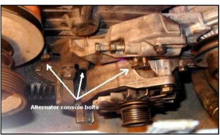
9 - Loosen console with alternator from engine - two 13mm and one 17mm bolt. This is to provide room to remove the center timing-belt cover. The "console" is a mount/spacer between the engine block and the alternator and power steering pump.
