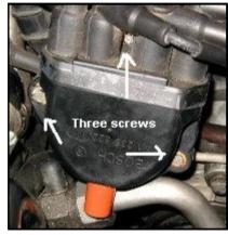
26 - Unplug all the wires (and the coil wire on the bottom) and lay back on the engine. Use a 4mm hex key on the plug wire loom at front/center of engine. Lay this section across the front of the intake manifold.
