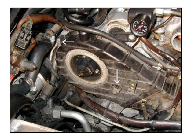
31 - For 5-speed cars (from the Workshop Manual p.15-105): "Remove clutch slave cylinder. Take off clamp on clutch hose holder and remove push rod. Let cylinder with connected line hang down." The two bolts are 13mm.
