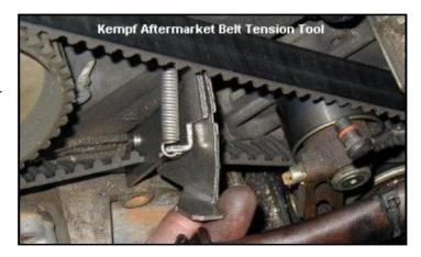
19 - Refill the tensioner with 90-weight gear oil by loosening the fill (left) and bleed (right) screws (4mm). The gear oil I bought had a nozzle tip and I was able to feed it into a 3/16" clear tube. The clear tube fit snuggly over the fill screw. By squeezing the oil container I was able to pressure the oil into the tensioner. It took about ten solid minutes to move 100mL (3+ ounces) into the tensioner before the bleed screw dripped. Tighten both bleed screws.
