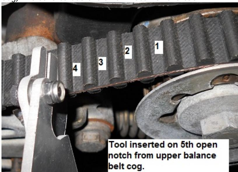
3. Gently press upward on the 9131-944 tool until the twist stop arm contacts the flange of the water-pump (slight adjustment of the twist stop arm angle may be needed).
