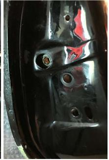
Remove the spacer using a large allen-head screwdriver. I haven't been able to locate this part in PET, but it is shown in the WSM as you can see below on the right:
