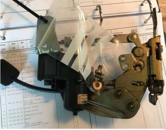
To remove the door handle and inner plate first remove the rubber cap of the front bolt. Next take out the two allenhead bolts that hold the door handle:
