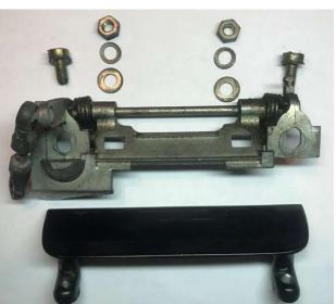
Remove the locking rod and bearing from the door. You'll first need to slide the end that's shown in the picture below out of the slot on the bearing. Then remove the two screws on the side of the bearing:
