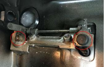
Remove the two hexagon nuts that hold the inner plate to the door (I know the allen-head bolts are not removed yet in the left picture.....let's call it artistic freedom...:-)...)
