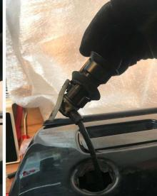
Release the locking rod from the door lock mechanism by pushing it out of the plastic cap:
