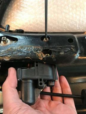
The door lock mechanism is now free so you can take it out. I stored it with the pan-head screws in a plastic bag tierapped to it...:-)
