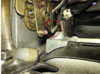
The door lock cylinder is still bolted to the door itself. To unbolt is first remove the small plastic cap and then unscrew the allen-head bolt. The picture on the right shows the spacer that sits in the door:
