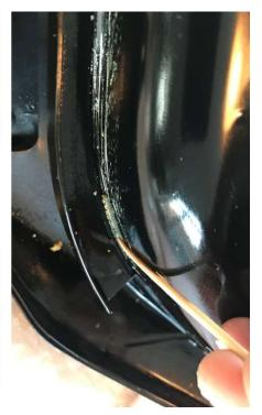
Another way to remove larger pieces of adhesive tape is a 'caramel disc'. I triw=e dit and it was very effective, not scratching the paint at all! The only downside is the huge amount of tiny rubber parts that come off the disc while using it:
