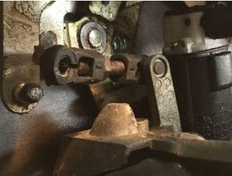
Push the black rod outwards (upwards in this picture, but remember my door is lying on its back). This will give you access to the white plastic operating rod that connects the lock mechanism to the door lock cylinder. Using the same tool is popped the rod of the metal ball:
