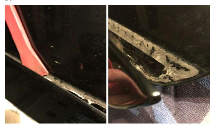
The disadvantage of the plastic tool instead of dental floss or a fishing line is that you do scratch the paint a bit; as my car will be painted I didn't mind:
