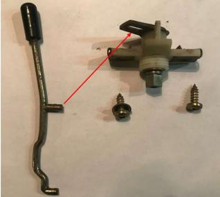
Last thing to do is to remove the door support from the door. Undo the screws and pull it out from the inside. Don't forget to also remove the rubber desk pad that sits between the door support and the door: it tends to stick to the door. Keep an eye on the curve in the door support, to prevent installing it the wrong way around:
