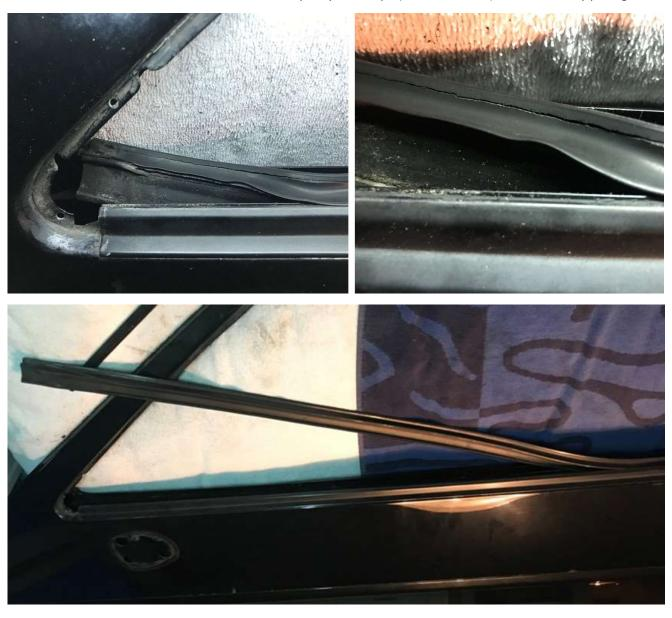
I then used the thinnest plastic tool I had to carefully tap the trim piece out, starting at the front and working my way towards the rear corner (and the bend in the trim piece):
