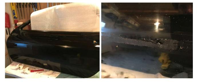
On the inside of the door was a lot of hardened glue, that could only be taken off by again using a lot cloths and of acetone. I spend hours on softening the glue en then very slowly removing it by rubbing with the cloth:
