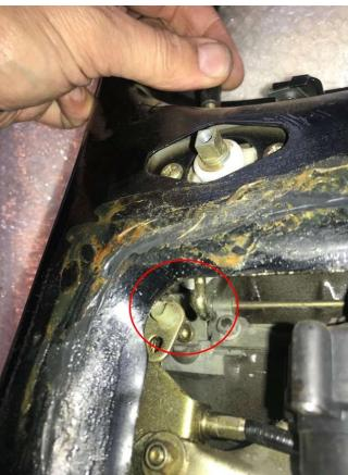
Remove the two pan-head allen-bolts that secure the door lock mechanism to the door. Keep them in a secure place: I haven't been able to find these in PET:
