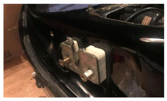
With the outer door lock out removed you can release the inner door lock mechanism from the door handle and the door lock cylinder. The picture below shows the door lock mechanism; on the left the bolt that held the security plate (that washer apparently becomes a challenge when re-installing the plate) and the on the right the connecting rod between the door handle and the door lock mechanism:
