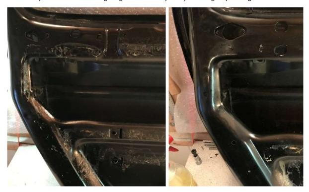
The picture on the left below shows some kind of bathroon sealant being used to keep the door seal in place.
