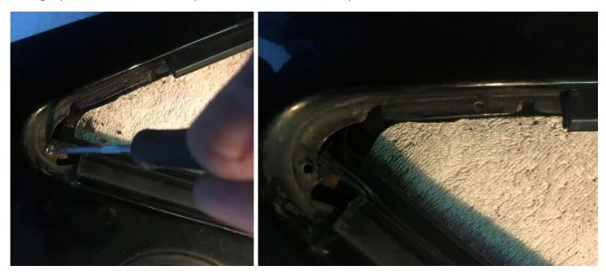
Next remove the upper trim piece (nr. 22). I first used a heat gun to heat up the trim piece. I then started above from where the filler piece was and used a plastic tool, tapping on it to get the piece off in that corner:
