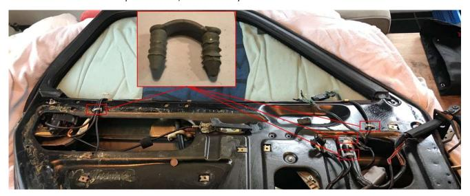
Remove the 4 clamps that hold the harness to the top of the door frame, as shown in the picture below:
