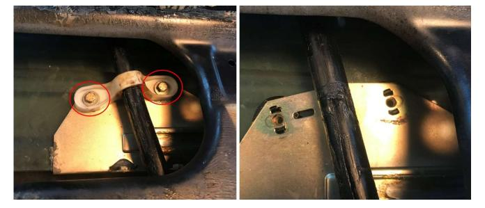
Unscrew the two allen bolts that attach the guide tube to the door frame. Then pull the guide tube free from the pin on the inside-bottom of the door:
