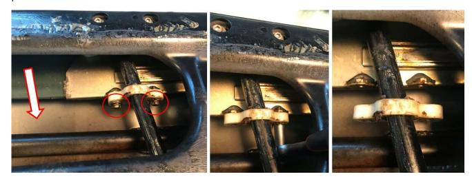
Slide the window down even further until you can see the two bolts that attach the upper slide to the window. Remove these bolts as well:
