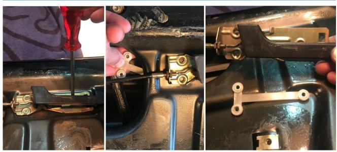
Unscrew the motor and lift mechanism by removing the 4 bolts shown below in the picture on the left. As I wanted to get the window guide tube out of the way as well before removing the motor and lift mechanism I put a towel below the motor to prevent any damage to the aluminum:
