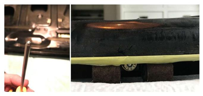
It took 3 days of drilling and numerous drills to finally drill a small hole in the bolt, enabling me to get a small metal hook behind the tip and force it out. Luckily the inside of the bolt was still in good enough shape to then use a regular allen-head screwdriver and remove the bolt.
