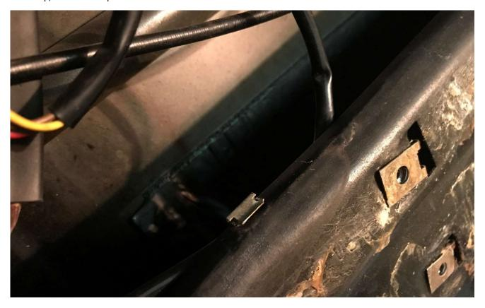
To take the door guard light out you have to reach inside the door and push the small plastic clips on the light housing. You can then just gently pull the housing of the bulb itself:
