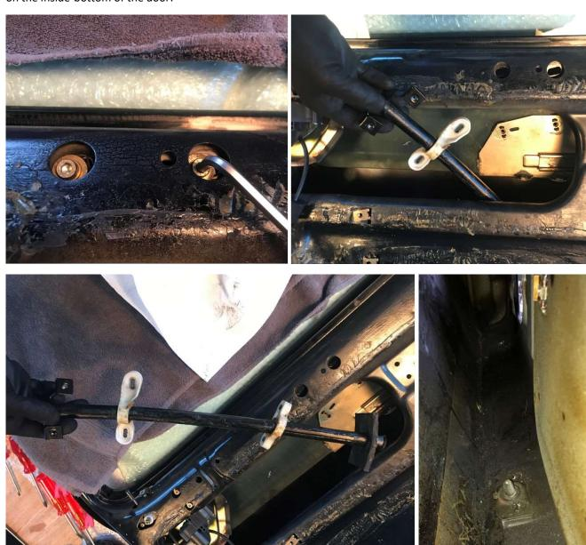
You should now have enough room to take the window motor and lift mechanism out through the opening:
