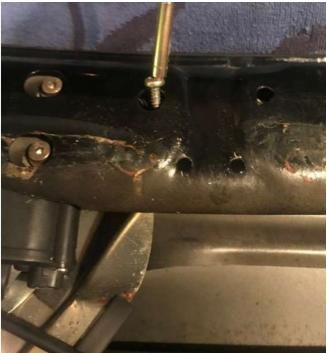
The security plate is held at the bottom by the bolt that attaches the reinforcement bar to the door frame. Loosen the bolt but DO NOT take it out: there is quite some tension on that bar, and it will be very difficult to get the bolt back in afterwards. When the bolt is loose, just slide the security plate out.
