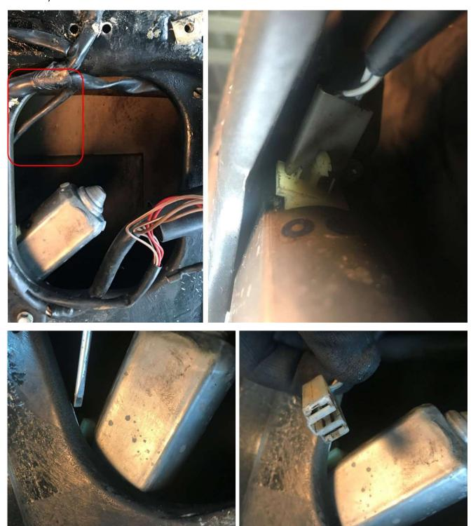
Last part of the harness to get out is the mirror harness. It disappears into the opening of the window motor and is held there by a small plastic clip:
