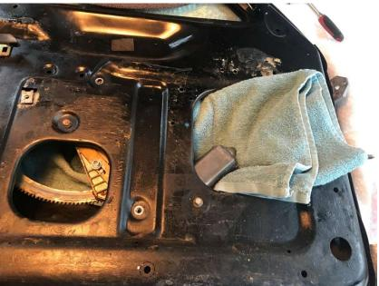
Move the motor and lift mechanism forward to free the roller from the guide rail. Lower them onto the towel and leave them there until the window guide tube is out:
