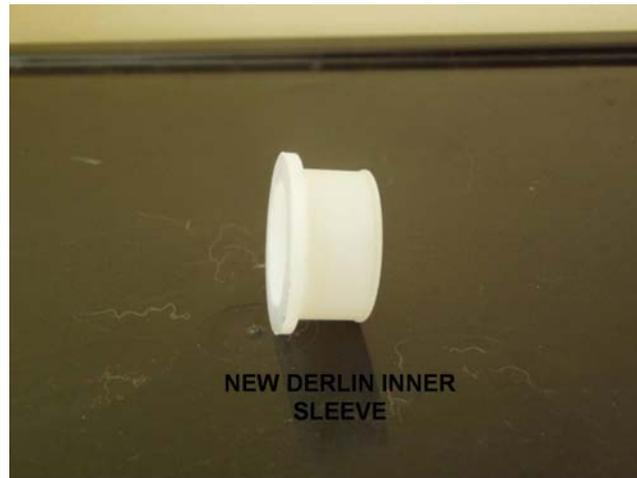
Material used according to machine shop was Delrin plastic. Do not use UHMW. It is too soft.
