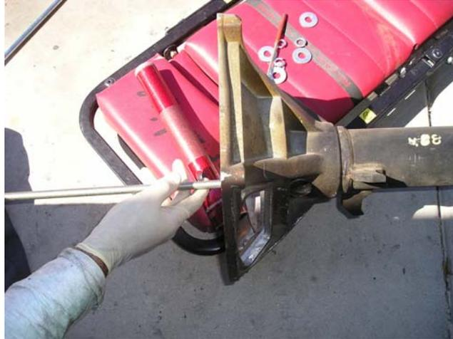
7. Put the go-cart pulley or the flat bar with 1" hole onto the protruding end of the threaded rod at the front of the torque tube. Add a washer and nut. This nut will be held stationary with a wrench. Alternatively, if you have a welder, you can tack weld the nut to the flat bar.
