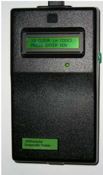
The tester then will start to initialise and test the next ECU – EZK (928 only) PSD, Tiptronic (964 only) and Heater ECU (964 only). The ECU's are checked in sequence, it is not possible to “skip” to the next ECU without reading the fault memory of each ECU in turn.
