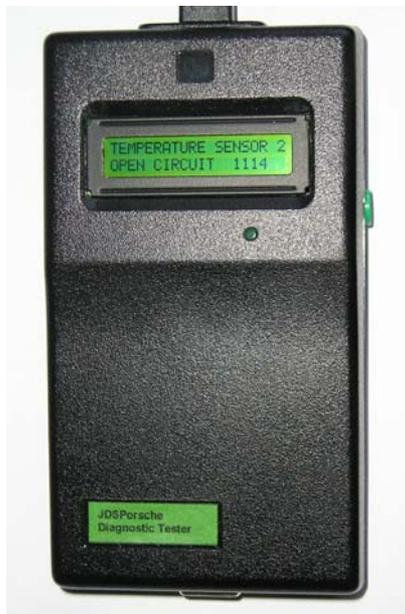
The tester will pause on each fault found, until prompted to continue. When all the faults on each ECU are completed, there is the option to erase all the fault codes and continue to the next ECU, or to retain them and to proceed. The displays **“ TO CLEAR LH CODES PRESS ENTER NOW”** and **“ TO RETAIN LH CODES PRESS ENTER NOW”** alternate until the required option is selected.
