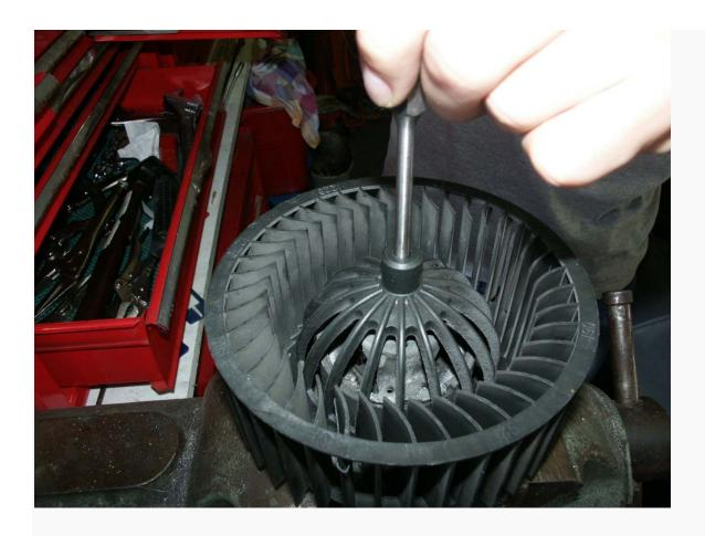
The shaft of the motor is a little longer, the fan needs to be pushed a little further an the shaft for clearance purposes.
