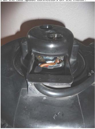
Separate the blower case halves by hand, and undo the 7mm screw holding the motor to the upper half - you'll note the slots in the case that allow the brush housings to fit in the case.
