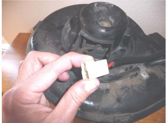
Pull the two spade connectors off the motor:
