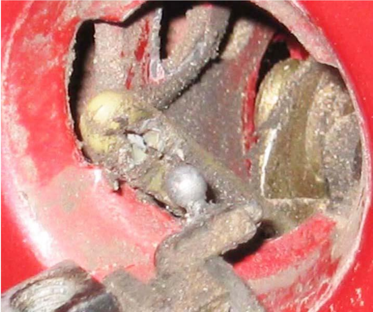
The below picture shows one of the pins that hold the core in the barrel
