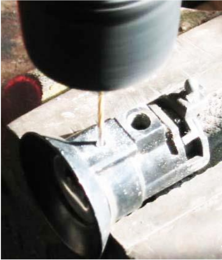
Using a diamond bit to erode the steel pin that I drilled off centre.
