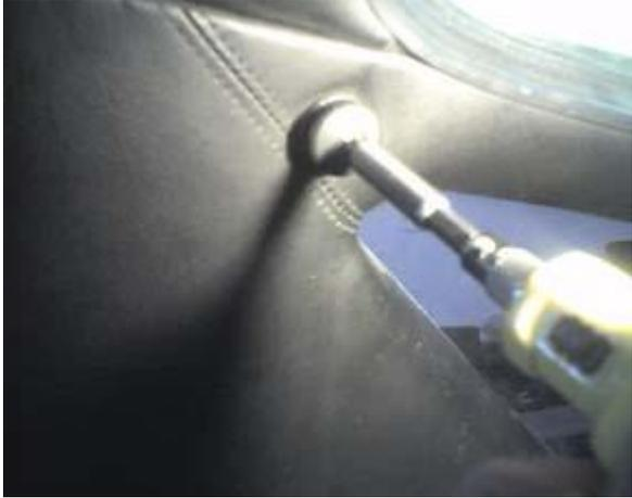
There are four screws that anchor the bottom of the panel and a 8mm nut at the end:
