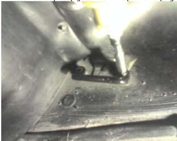
Now that all the screws are out, it's time to pop out the pegs. There are three that hold the panel to the C pillar. I inserted a bone tool between the top of the panel and the C-pillar, holding the tool horizontal and then pulling down on the end. The pegs make a firm pop as they let go:
