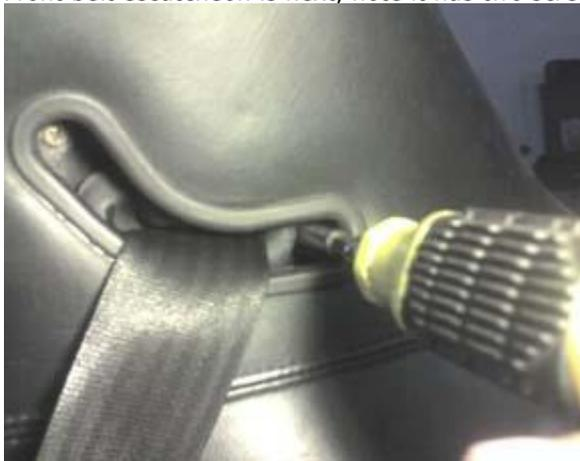
There are two screws above the front seat belt anchor on the B pillar.
