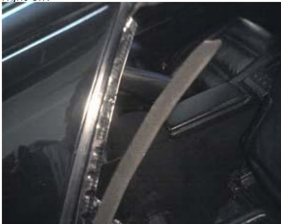
The tool kit tray stay gets in the way when trying to remove the panel, and should be removed:
