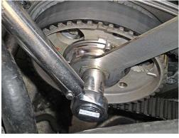
Torque cam bolt to 47 ft. lbs. (65 Nm) with torque wrench. (Use wrench to counter hold hex washer.)
