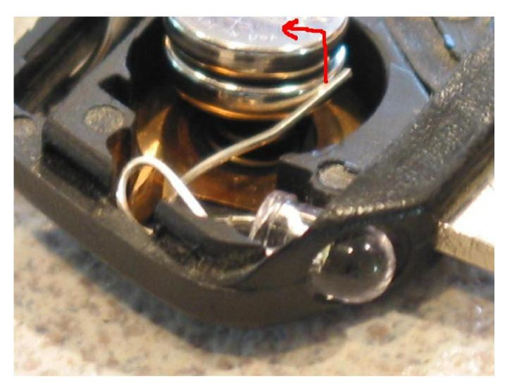
Next, balance the cap on top of the batteries and pole. The pole should be sandwiched between the cap and batteries. Just get it to stay, it wont be secured until you close the whole key. Its a little tricky, as the batteries teeter a bit on the spring. Just try to keep it all together. Once its closed up, it will stay. (just make sure that pole IS ontop of the batteries when you close it up.
