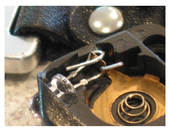
Third, place the two batteries on the spring. Positive side up. The long LED pole should be placed ONTOP of the batteries. I had it to the side in the picture because it wouldnt stay without the cap on. When you assemble it, the pole has to be ONTOP of the batteries. If its to the side, it wont work consistently.
