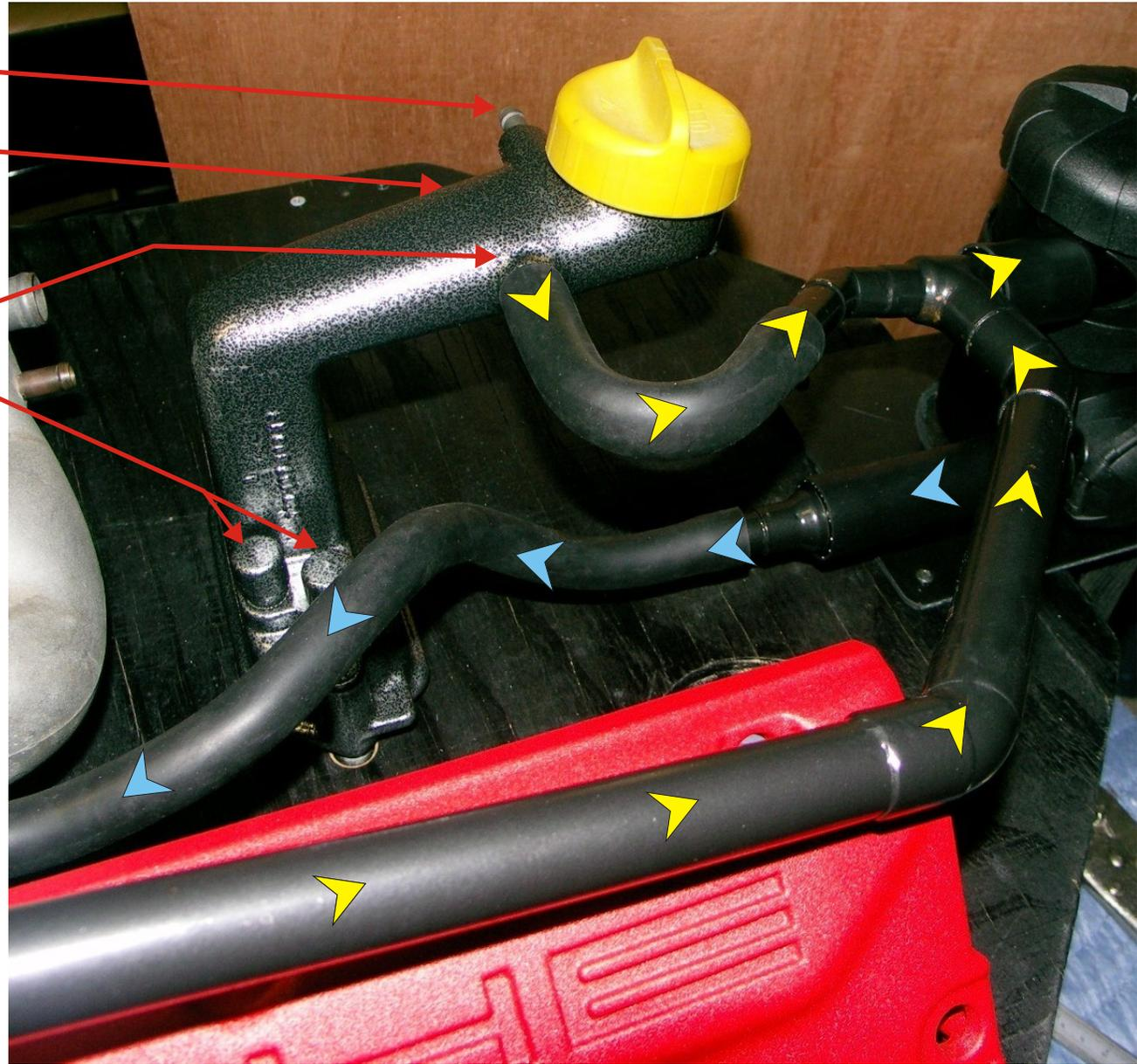
➤ = Oil & vapors flow from rear PS cam cover elbow & crank case to the Provent oil separator
