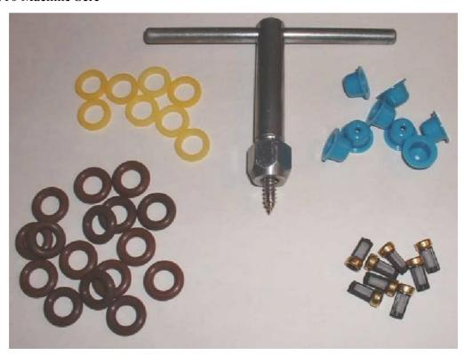
Use the #10 machine screw to remove the internal filter from the injectors.
