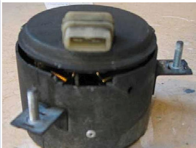
Place holding tabs back in position. I used a cold chisel for this.
