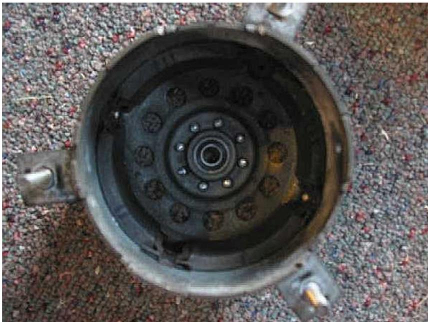
Reassemble rear plate onto motor with brushes retained. Remove nails. If you only just put the nails through the top hole on the brush housings they are very easy to remove.
