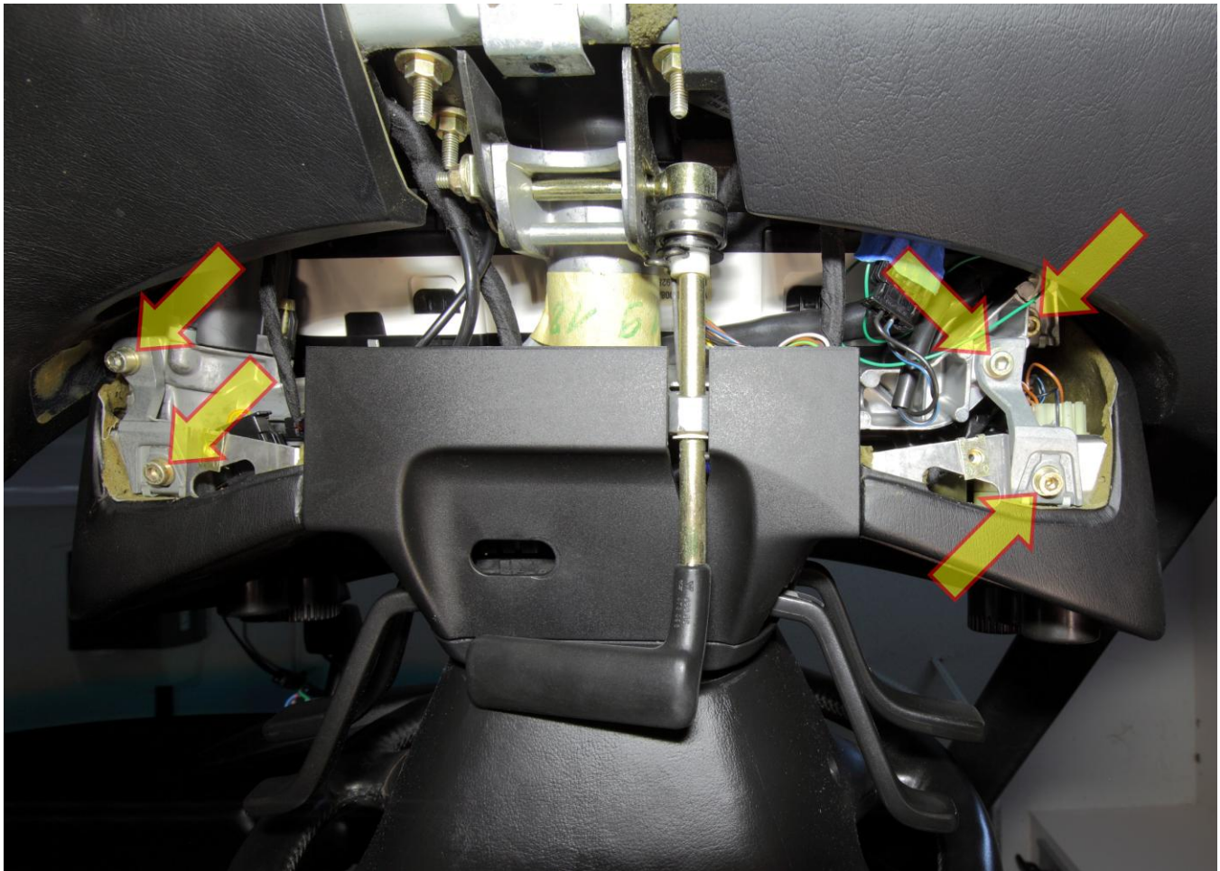
Figure 1 Looking up at the bottom of the instrument pod and the five screws that secure it
