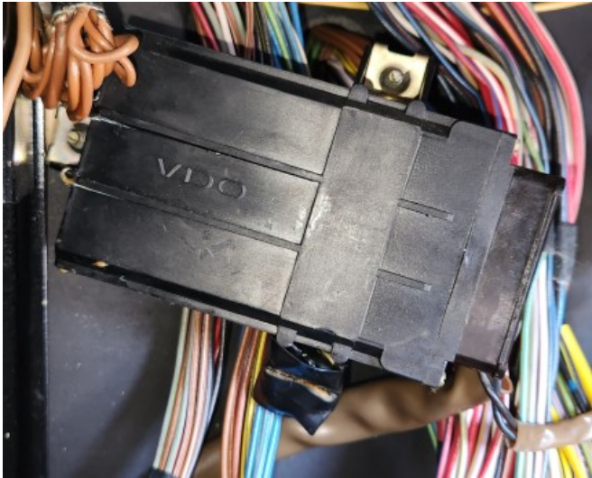
928.641.503.02 lamp controller located above fuse/relay panel
