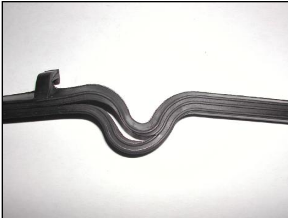
Photograph of RHS of Oil Pan Gasket showing split
