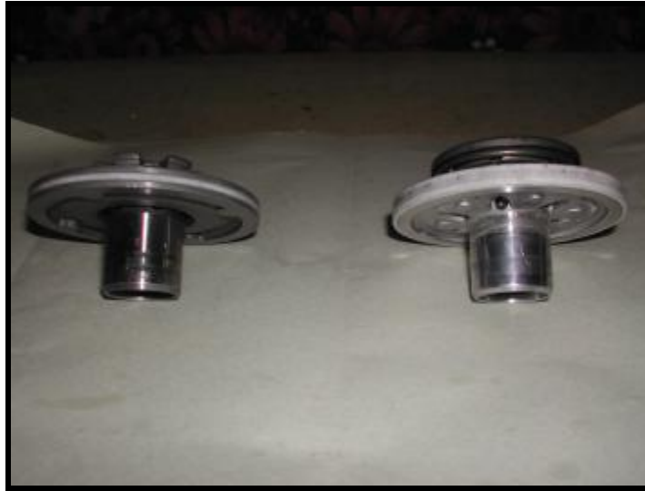
Old B2 Piston Assembly on LHS & Modified B2Piston Assembly on RHS
