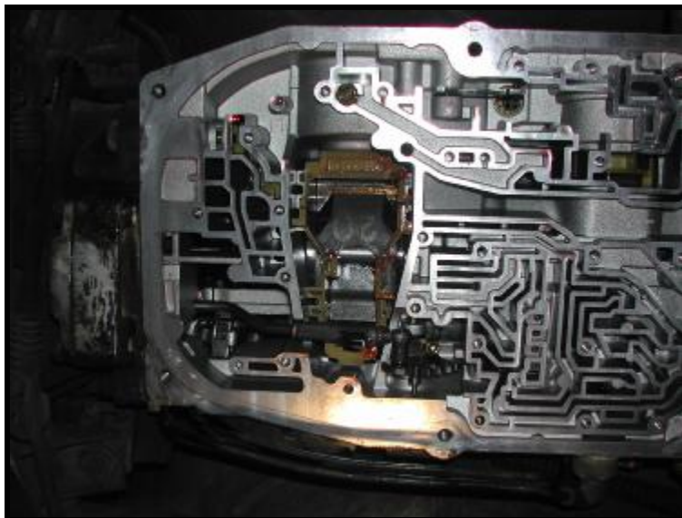
Transmission with Valve Body, (Lower Cover & Intermediate Plate removed) showing Brake Guide and B2 Brake Band The leaf spring set bolt hole and locating pin hole can be seen adjacent to the lower transmission case edge, to the upper left of the flash reflection
