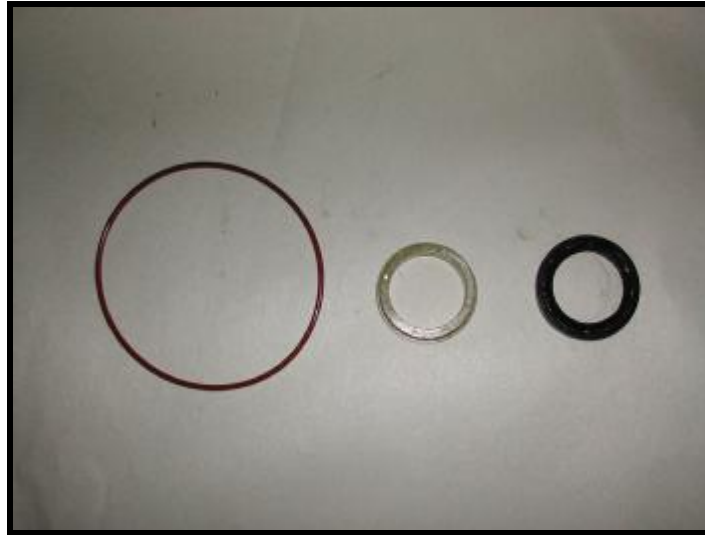
B2 Brake Band Piston Cover “O” ring, Piston Assembly Bush and lip seal
