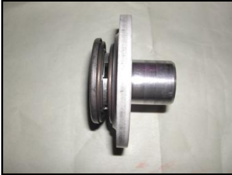
B2 Brake Band Piston Assembly with a view of retaining washer, spring, "T" plastic seal ring and OD of piston cylinder where lip seal seals
