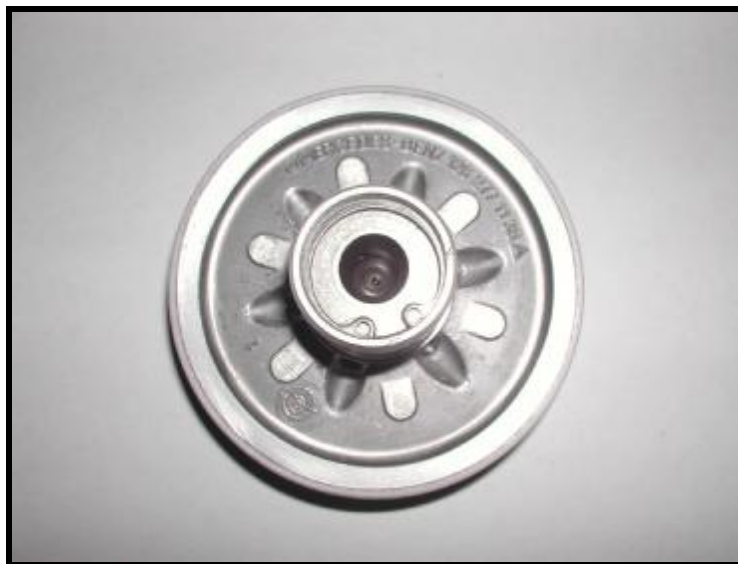
B2 Brake Band Piston Assembly With a view of thimble piece and retaining circlip
