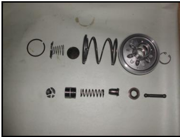
B2 Piston Assembly damage
