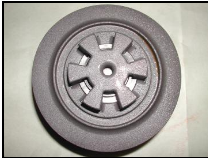
B2 Piston Old model Piston Assembly appears to be cast iron
