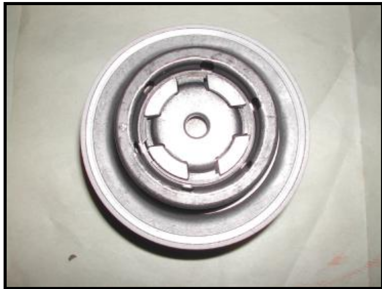
B2 Brake Band Piston Assembly with spring retaining ring, circlip and cruciform piece holding the conical spring and non-return valve that can be seen through centre hole
