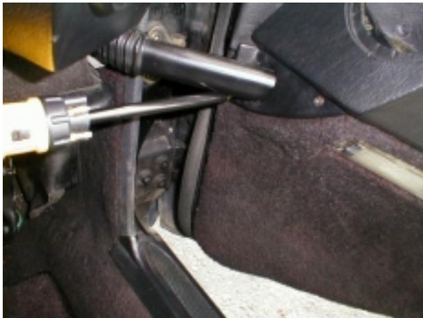
1. Remove the two screws holding in the [triangular piece](#) at the front of the door, where the wires enter. One screw is easy to see in the photo, the other is hidden, but the screwdriver is pointing at it. Once the screws are out, pull the triangular piece down a little (it wedges up under the armrest), and then back, like [this](#).
