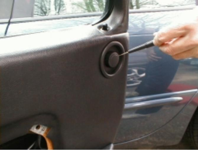
4. Now the doorlock knob needs to be removed. First [pry off the cover](#) over the knob with a thin screwdriver (or something similar).
