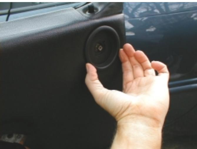
It just [screws](#) out. The center of the backing is threaded. If it is hard to get started, you may need to find something that you can insert into the notches in the backing to turn it (I brightened the previous photo some so the notches are more visible).
