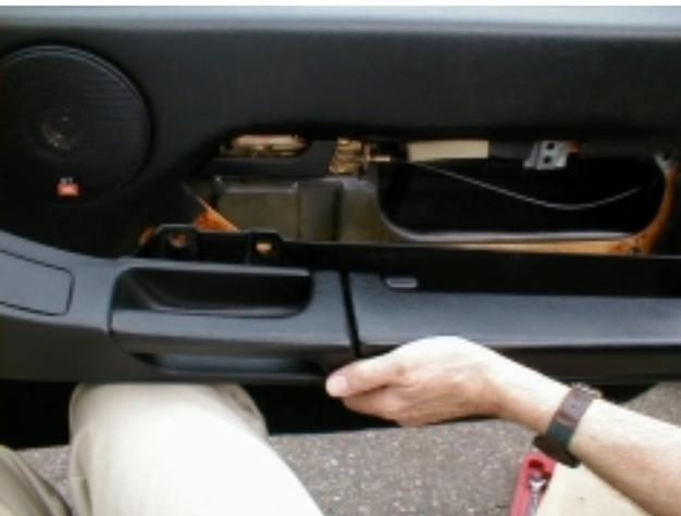
6. Once all of those bolts are out, you can pull the armrest off. It should just [lift right up](#). This is on the passenger's side panel,
