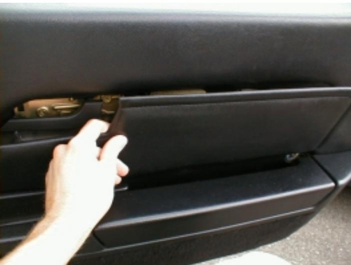
3. Now remove the door panel [insert](#). It's held in at the top by white push-in clips, as well as being pushed down over the armrest. So first pry the upper rear portion away from the panel (the clips are both on the tip, one at the rear, one in the middle). Once both clips are out, then pull the insert upwards. In the photo, the clips have been pulled out of the panel (they should stay in the insert), and it is about to be pulled up.
