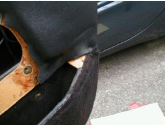
7. Then remove the [screw](#) at the rear of the panel (already removed in photo), at the base of where the armrest sat. There may also be another screw somewhere along the bottom of the door panel (I seem to recall one), but if there is, it is missing in my panel. Before proceeding to the next step just look around and make sure there aren't any other screws in the carpeted portion of the panel.
