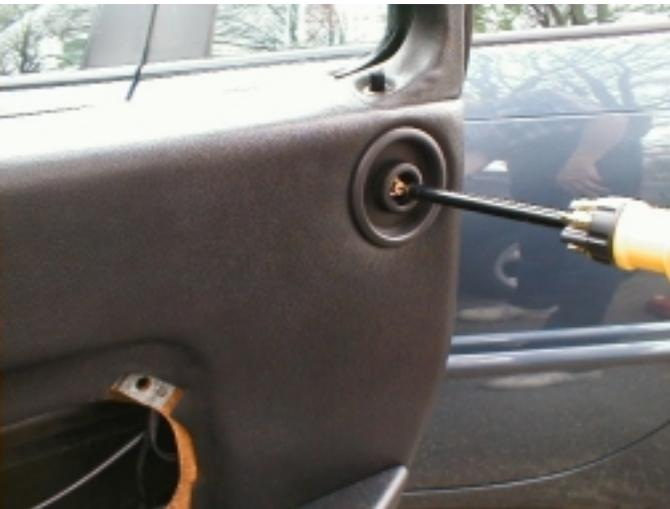
This will reveal a [screw](#) which holds the knob in. Remove the screw, then pull the knob straight off. Next the knob backing needs to be removed.
