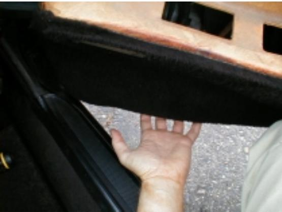
Work your way [around](#) the edge of the panel, prying it away from the door (the clips "pop" in and out). In addition to the clips, the panel is held in at the top where it pushes down into place.
