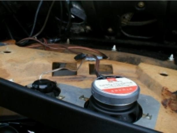
9. To pull the panel off the door, you need to pull the black plastic [wire holder tube](#) through the hole in the front of the panel.
