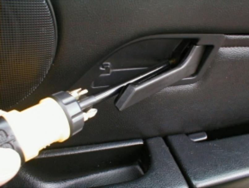
2. Pull the door handle to reveal a [screw](#) behind it that holds in the door-handle backing. Remove this screw, and [pull the backing off](#) over the door handle.
