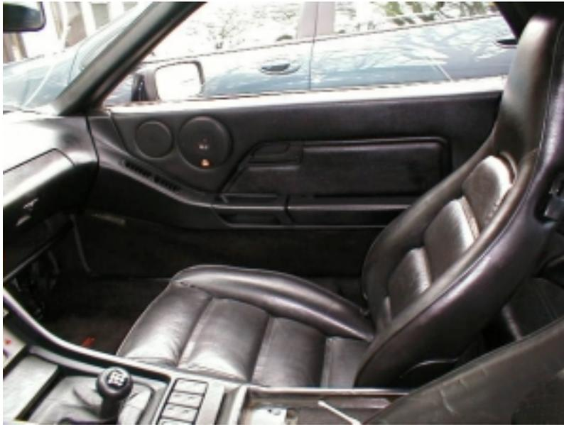
Now, let's go through the removal of the door panels, step-by-step. Some of these steps (the initial ones at least) can be done in various orders, but the big pieces need to come off in this order. I find the best way to do this is to have the door partially open, and to sit on the edge of the car next to the seat.
