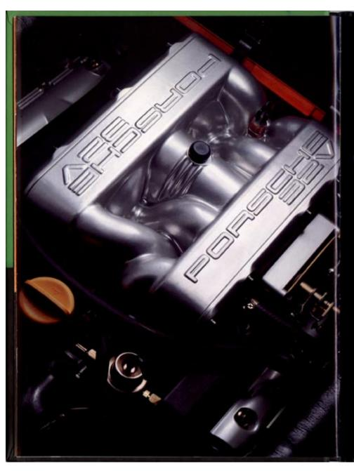
The heart of the Porsche 928. The light alloy V8 engine features 32 valves and 4 overhead camshafts. The 5.4 litre cubic capacity of the 928 GTS produces 350 bhp (257 kW) of performance and a torque of 500 Nm at 4250 rpm.
